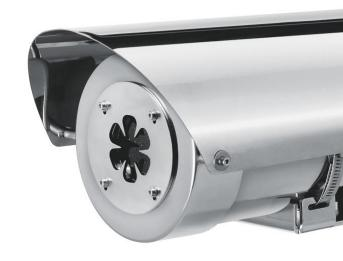
Workswell SAFETIS EX-proof camera offers great resolution of 640 x 512 px, sensitivity of 50 mK (0.05 °C) and fast response within milliseconds. The powerful communication interface allows connecting SAFETIS camera directly to any computer via Web-server or directly to SAFETIS Control Unit via Ethernet RJ45. The SAFETIS camera has integrated 7 digital outputs in the camera and 7 digital outputs in SAFETIS Control Unit that can be triggered at the same time if needed.
